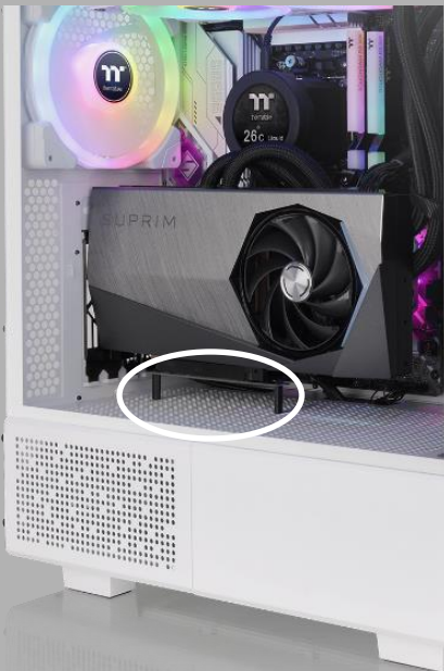
Supports 90° riser cable installation
