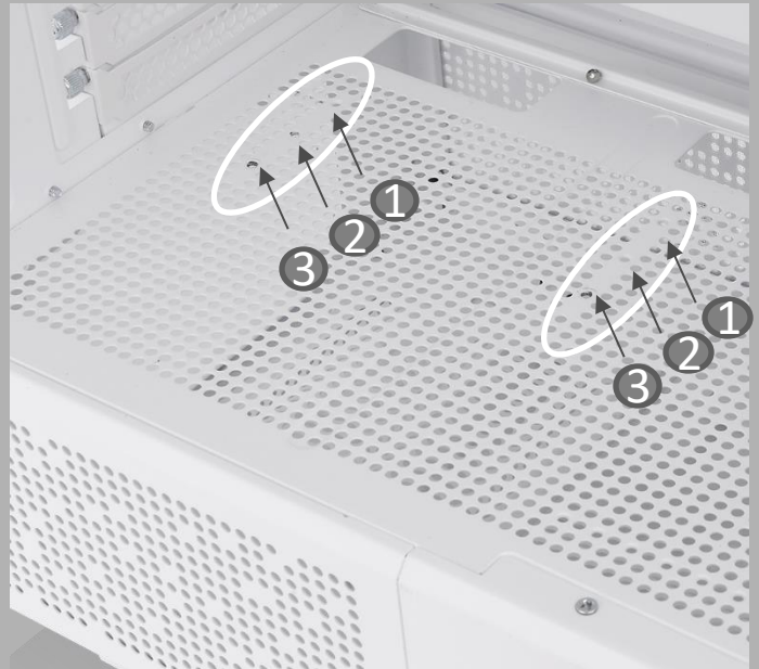
Three places for riser cable installation
